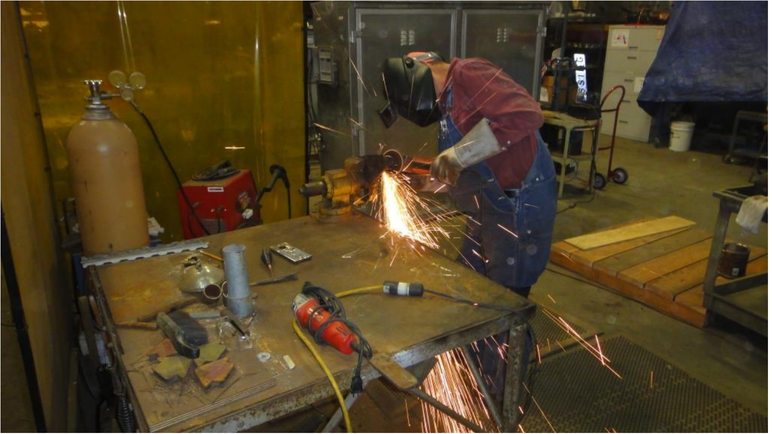
Cliff using the grinder on the new foot of the derrick crane's support strut
