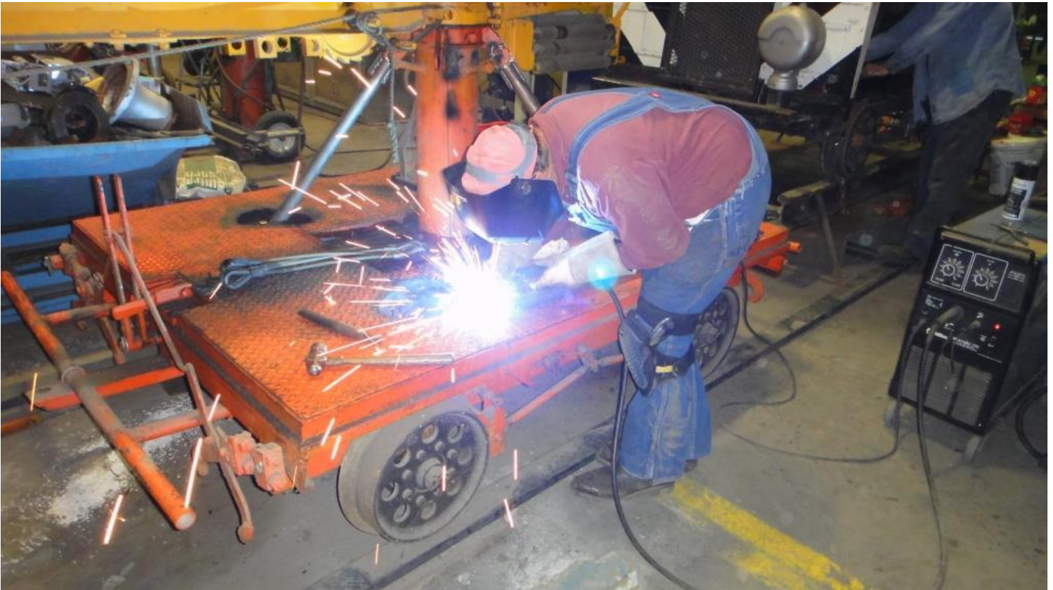
Cliff welding the strut-foot in place
